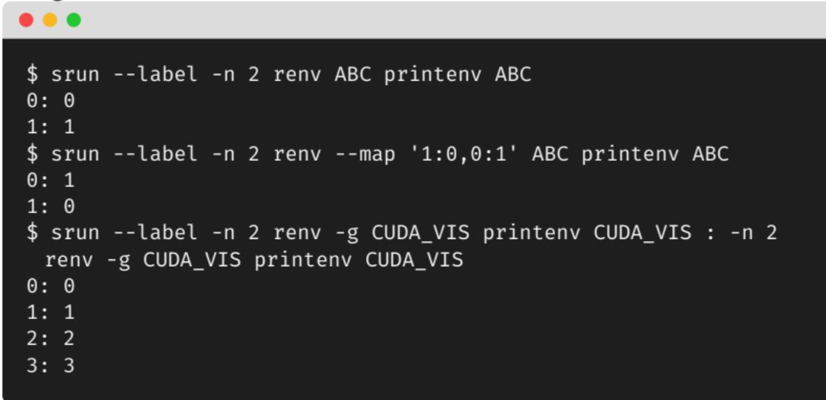
A screenshot of a terminal window showing three command examples. The first command runs two processes with rank IDs 0 and 1. The second command uses a map to swap the rank IDs. The third command runs four processes with rank IDs 0, 1, 2, and 3.
